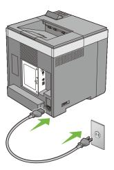
2 Turn on the printer. When the printer is connected via a USB cable, the USB driver is automatically installed.
